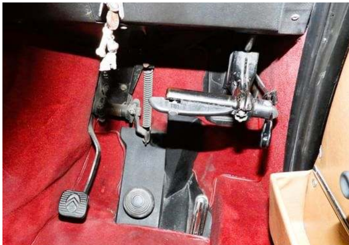
The clutch, brake, accelerator and hand brake. The brake is a button, when pressed hard the car will come to a complete stop.
