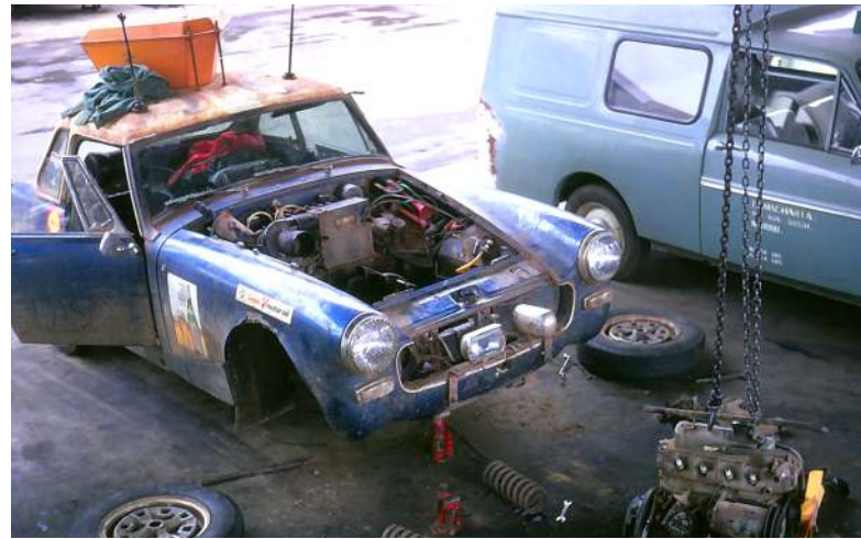
Welding up the MG front suspension in Nairobi. The engine had to be taken out
