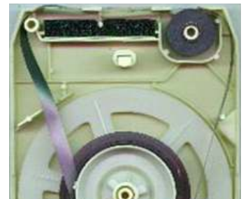
Inside of an 8-track tape. The tape is pulled off the inner part of the reel then fed back onto the outside, giving continuous playing
