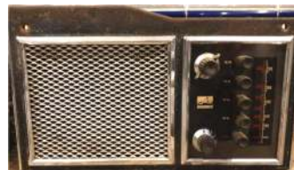
His Masters Voice valve radio from a Rover P4 90. Stealing 4 amps at 12v when the amp was just idling
