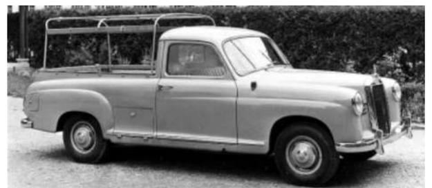
*Binz version of the Mercedes with integrated pick-up body, shorter cab and access to the spare wheel under the load-bed*
