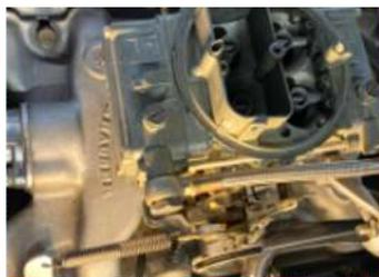
*Carburetion is via a 4-barrel Holley 390 CFM 'Double Pumper' with Offenhauser 360 deg manifold which allows the carb to sit lower on the engine, giving space for the bonnet to close.*
