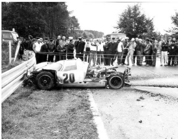
*The wreck of the radio-controlled 'Porsche 917'. Thanks to the missing rear clip, the Lola T70 MKIII B chassis, stock block Chev V8 engine and Hewland LG600 gearbox can be seen. Oops!*
